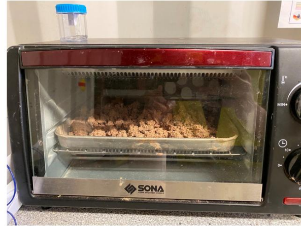
Heat excavated material at high temperature (250°C) for 1 hour to dry out the mixture
